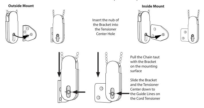
While holding the lock firmly in place, check that the loop can move freely through the Tensioner
