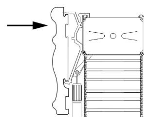
Press the top forward firmly until the Valance snaps into place
