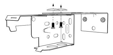
Using the nuts and bolts provided, attach the Mounting Brackets securely to each Extension Bracket
