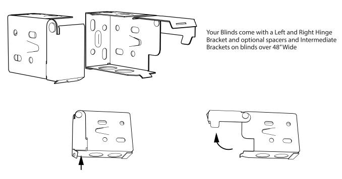
Open Brackets by pressing against the locking tab on the bottom of the Bracket and swinging open
