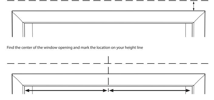
Mark lines at half the ordered width from both sides of the center line to determine bracket location
