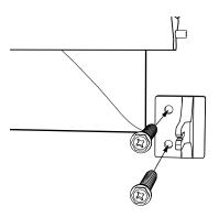
Raise the Blind out of the way and secure Hold Down Bracket to wall with two screws
