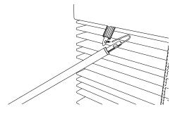
Wand installation is complete when Locking Collar is fully seated
