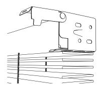
Close each Hinge Bracket until the locking tab is fully protruded through the locking hole
