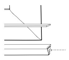
Fully lower blind and mark Hold Down Pin location
