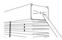
If your Headrail is Loose in the Brackets, use a screwdriver to pry the tabs of the end caps out
