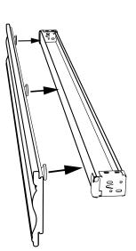
Press the forward firmly until the Quick Clip snaps into place on the Headrail Clip
