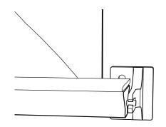
Push pin into Hold Down Bracket in a position that the blind still rests comfortably
