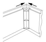
Slide Returns and Valance together until a flush corner is made
