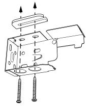
Line up the slot in the Spacer with the holes in the Bracket and use two screws to attach to window opening
