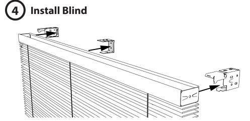
Center Headrail and insert into the mounted Brackets
