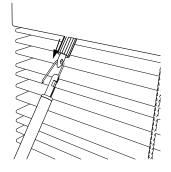
Insert the Hook of the Wand into the eyelt of the Wand Control Arm
