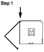
Tilt fascia so that the lip at the top of the fascia can rest into the slots in the top of the bracket
