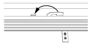
rotate Cam Bracket arm counter-clockwise until fully seated against track to lock in
