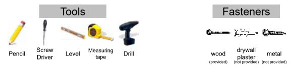
All bracket mounting screws must screw into wood. If the installation requires mounting the brackets to a surface other than wood, be sure to use the appropriate fastener
