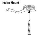
Screw Swivel Bracket directly into mounting surface
