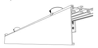
Rotate Cam Brackets counter-clockwise to lock in the valance and the track
