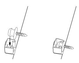
Insert a Button Screw at each Button Catch
