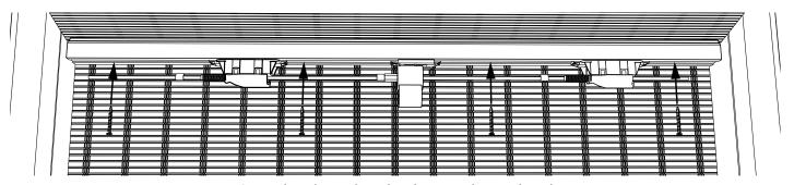
Screw directly into board and up into the Head Jamb
