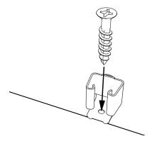
Use a screw to secure the Button Catch at each location
