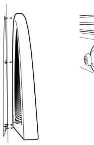
Press the Arch against the Button Screws to mark the locations of each screw
