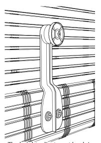
The height adjustment knob is located on the back of the shade
