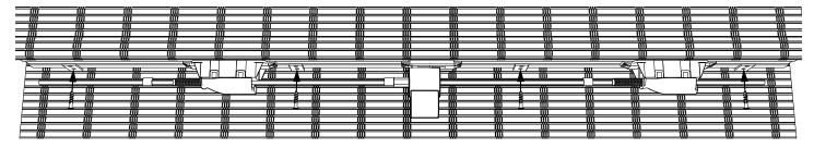
Secure headrail to brackets using provided screws from underneath
