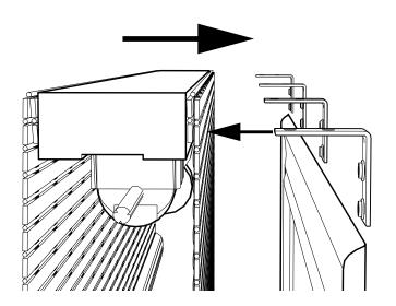
It may be necessary to cut material or liner to get the bracket through
