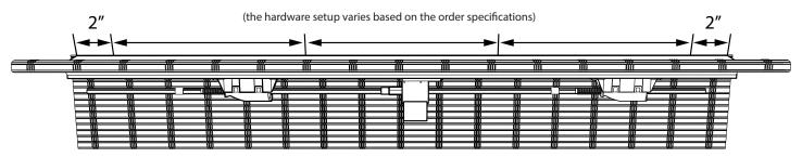
Evenly space remaining brackets or screws without interferring with hardware, cords, or vertical strings
