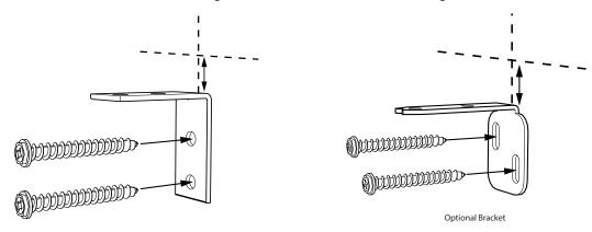
Install the Brackets with 2 screws into the mounting surface
